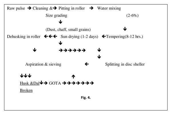
Fig. 4 Process for dehulling of Bengal gram
