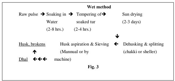
Fig 3 Dehulling of tur- wet method
