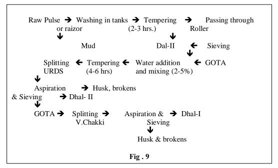
Fig 9 Process for dehulling khesari pulse (lakh)
