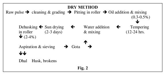
Fig 2 Dehulling of tur- dry method
