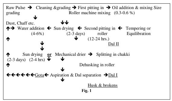
Fig. 1 Dehulling of tur-large scale
